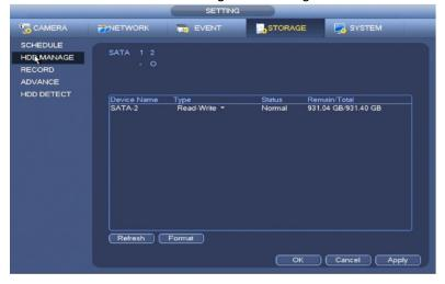
Check the status section, it should be normal. If it has an error, you can attempt to format the drive, which will erase any footage, but may resolve the issue.
