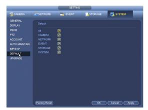
Simply login, Go to **Main Menu > System > Default.** Select Factory Reset to reset device to default settings.
