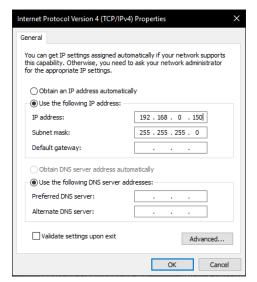
Enter in your IP address. Click in the subnet mask field and it will generate one, you can leave the gateway blank.
