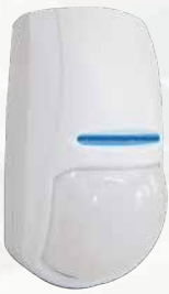
15m PIR sensor, dual pyro, tamper, N.C, incl. brackets
