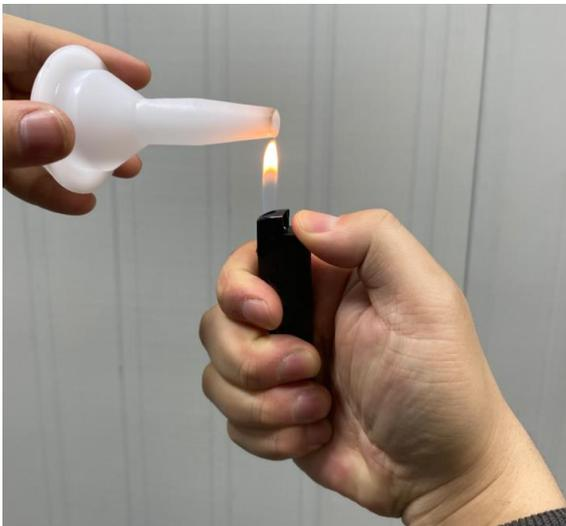
2. It is recommended to use a lighter to heat the tip of the rubber nozzle for about 2s to prevent it from springing back after being flattened.
