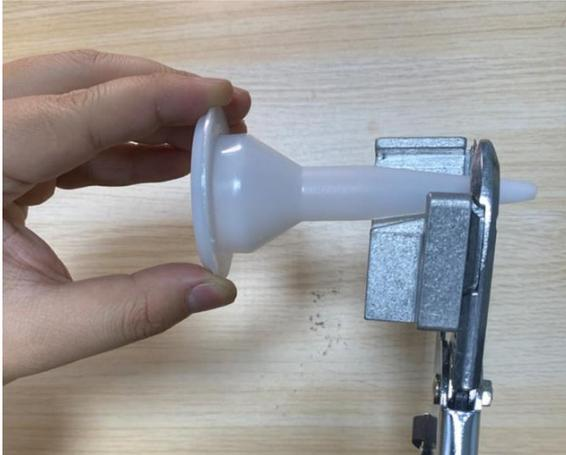
1. Use a straightedge or tape measure to measure the length of the head of the nozzle 20mm, confirm the cutting position, and then use the tool to cut in addition.
