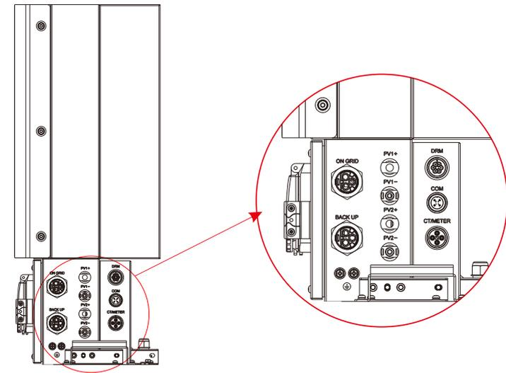
Figure 13 Cable Box Bottom View, Wiring Connectors
