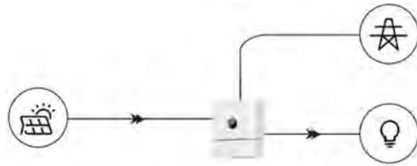
• **SELF CONSUME (with battery):** The energy generated by the solar panels will be used in the following order: Feed the home loads; Charge the battery and then, feed into the grid. When the solar panels are not producing power, the load will be supported by battery to enhance self consumption. If the power supply from the batteries is not sufficient, the grid will support the load demand.
