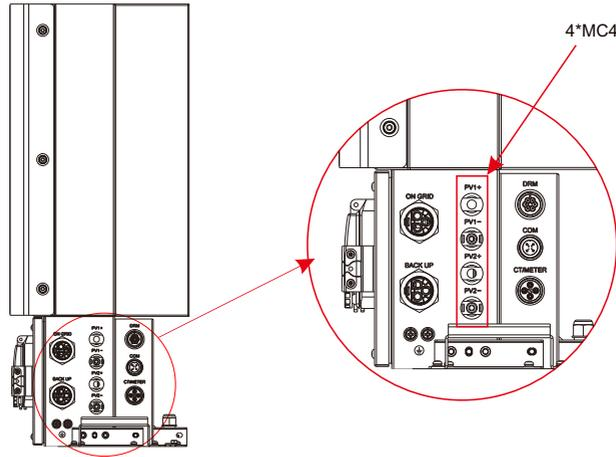
Figure 16 PV Wiring
