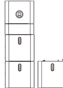
Figure 18 Increase the Battery Modules
