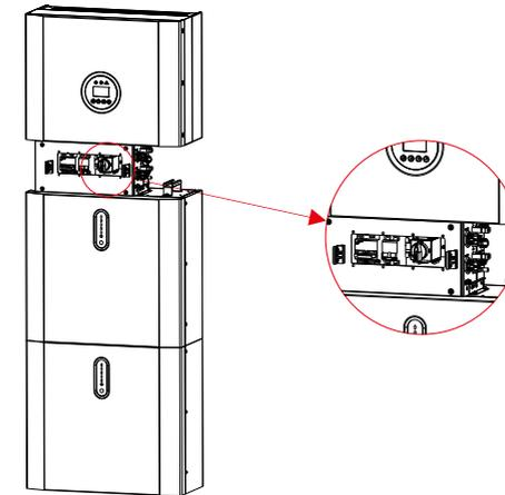
**Step 1:** Turn on the external PV switch.
