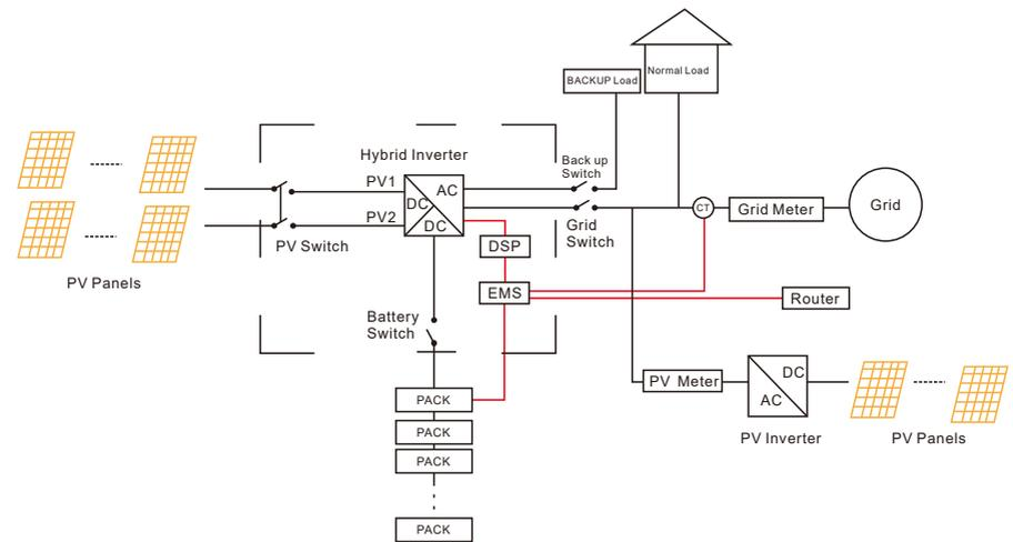
Figure 23 Hybrid-coupled system
