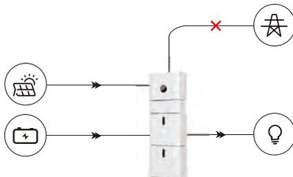
• **PEAK SHIFT:** This mode is designed for time-use mode customer. The customer is able to set up the charging/discharging time & power via inverter screen or APP.
