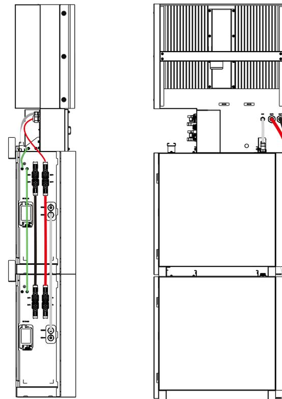
Figure 15 Wiring the Battery Power Cable
