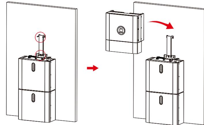
Figure 10 Inverter Installation
