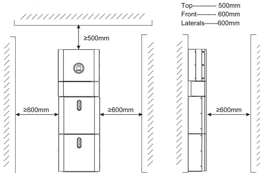
Figure 8 Limited Distance of Installation to Neighboring Objects
