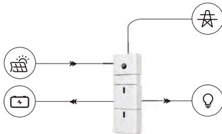
• **BAT PRIORITY (with battery):** Under this mode, the battery is only used as a backup power supply when the grid fails and as long as the grid works, the batteries won't be used to power the loads. The battery will get charged with the power generated by the solar panels or from the grid.
