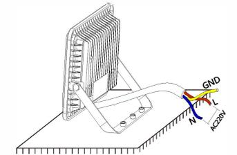
3-Only use a round cable supplied to connect this fitting.(6mm Diameter minimum)
