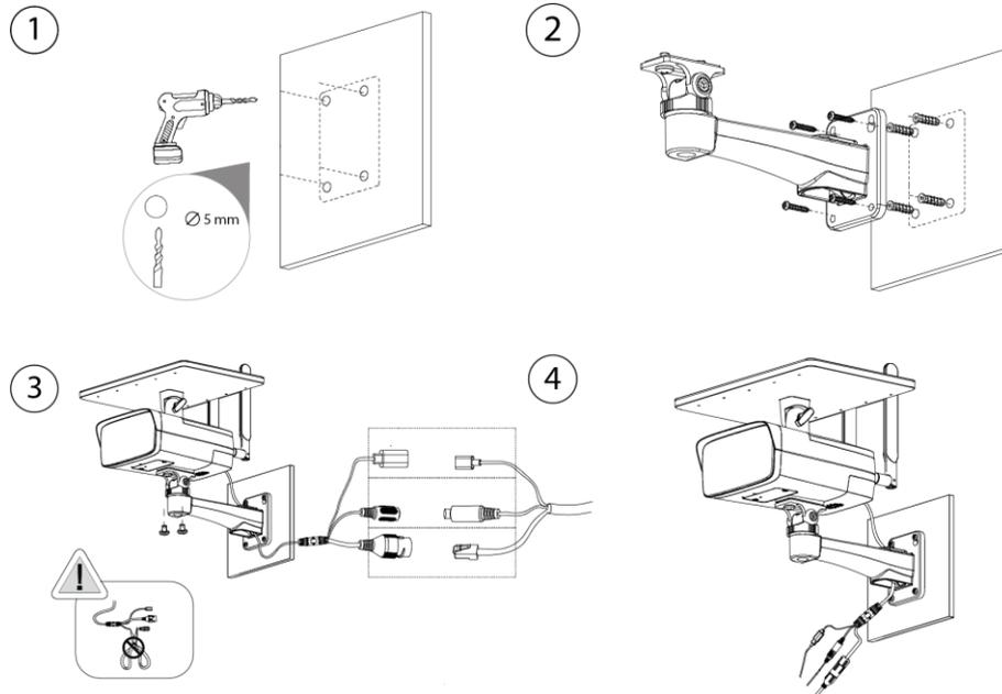
Figure 3-7 Cable going through the mounting surface
