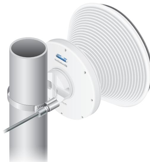
*Pole-Mounting of the IsoStation 5AC*
