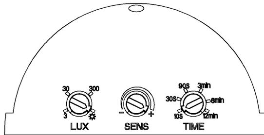
**Note: when testing in daylight, please turn LUX knob to (SUN) position to allow the sensor to work.**
