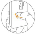
Press the black button on the rear of the motion sensor.
