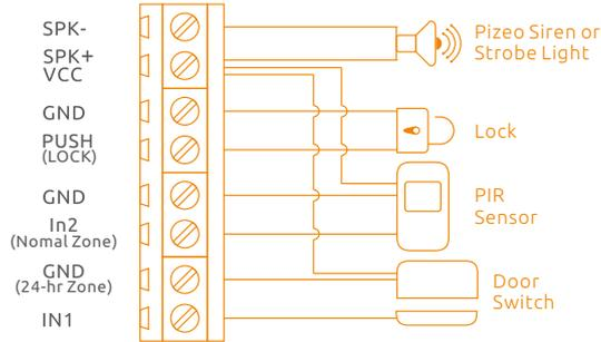
1. Connect one wire to IN1 or IN2 block while another to GND block. If no power supply is needed for wired sensor, don't connect to VCC terminal.
