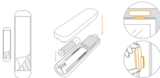
Recommended installation for gap between moving part and frame
