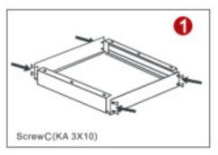
Assemble the four frames with Screw C to a whole square.
