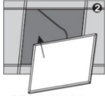
1. Remove the plasterboard from the ceiling. 2. Fix the panel into ceiling.
