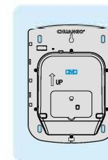
Drill four holes and fit the wall plugs, and then fit supplied fixing screws in the holes.
