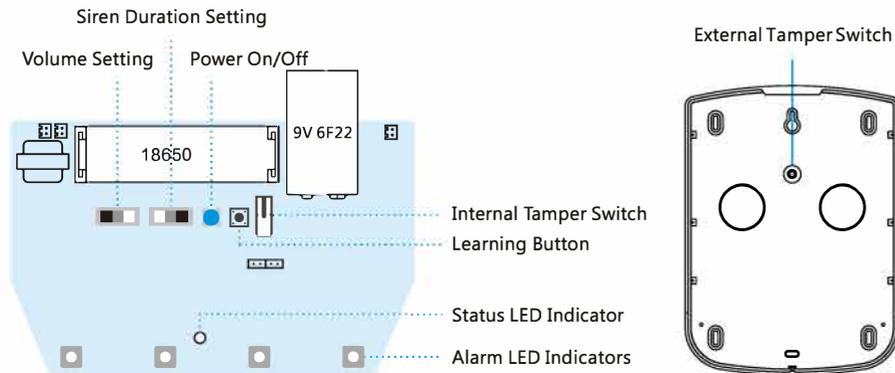
**Note:** The status LED will flash once every 5 seconds in arm status. It will not flash when in disarm status. The siren will sound immediately if the tamper switch is triggered.
