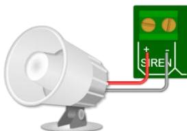
The siren connects directly to the siren output and can drive up to a 30 watt siren.
