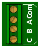
The connector labelled A, B, C and Com connect to the corresponding connectors with the same label on the Monitored Power Supply.
