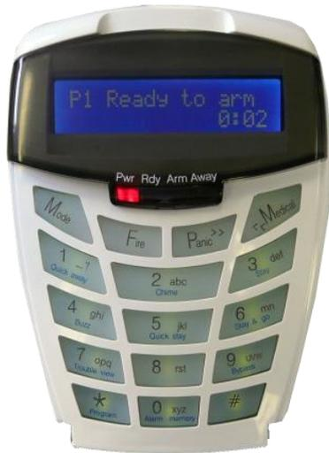
Liquid Crystal Display Keypad (LCD)
