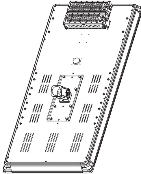
**Note:** The solar panel and light have two separate angle adjustment points. More precise angle configurations can be made by adjusting both.
