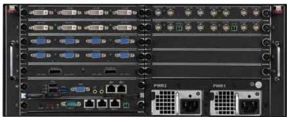
Above: VSVIDEOWALL with optional cards & PSU; base model differs in appearance
