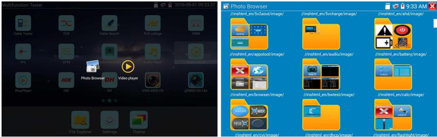
The Media player can browse video and image files. It supports the video formats of MP4, H.264, MPEG4, and MKV. The Integrated Mount Tester recorded files can play directly via the Media player. The Media player will automatically display the video files from the tester Click on the desired file to play. Click RETURN to exit.
