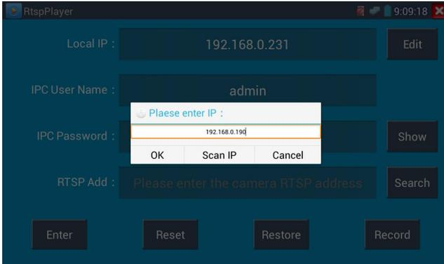
**Local IP:** This is the Integrated Mount Tester's IP address.
