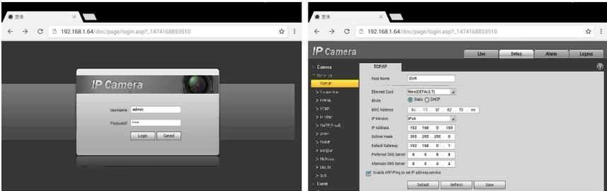
The IP camera and the tester be on the same network segment for the browser to interface with the camera. If they are not in the same segment, click the button
