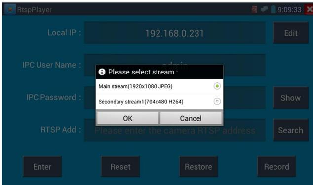
Note: In the event the Integrated Mount Tester does not auto detect the rtsp stream, refer to the specific camera manufacturer for the specific rtsp stream url. you may find this on line with a search of the camera model number and the word rtsp.
