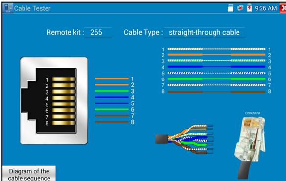
Test LAN cable or telephone cable.
