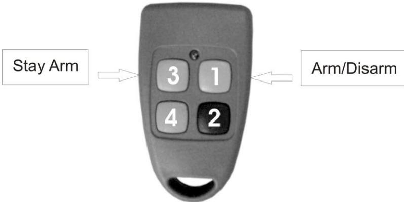
The functions that can be assigned to a button are: arm/disarm, stay, relay 1, and relay 2. Each button can be assigned multiple functions, or no function. It cannot be assigned both arm/disarm and stay. Different buttons can be assigned the same function.
