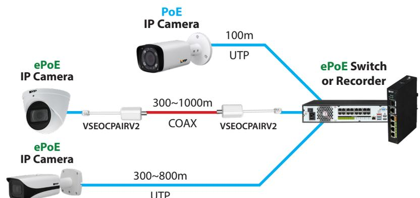
Note: Both an ePoE camera **AND** an ePoE NVR/switch are required for long distance Power over Ethernet transmission.
