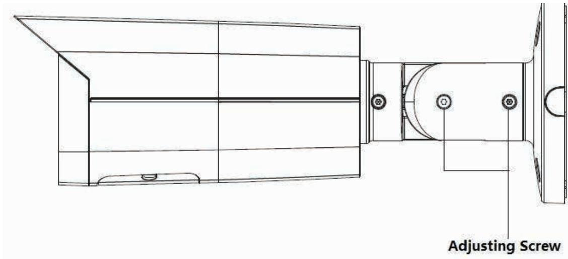
1. Use the screwdriver found in the accessories bag to loosen screw.
