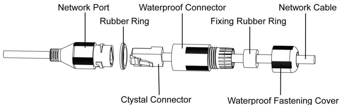
1. Install the rubber ring into the network port, keeping the smaller hole of the rubber ring facing outwards and fixing the rubber ring onto the main body of the waterproof cable.
