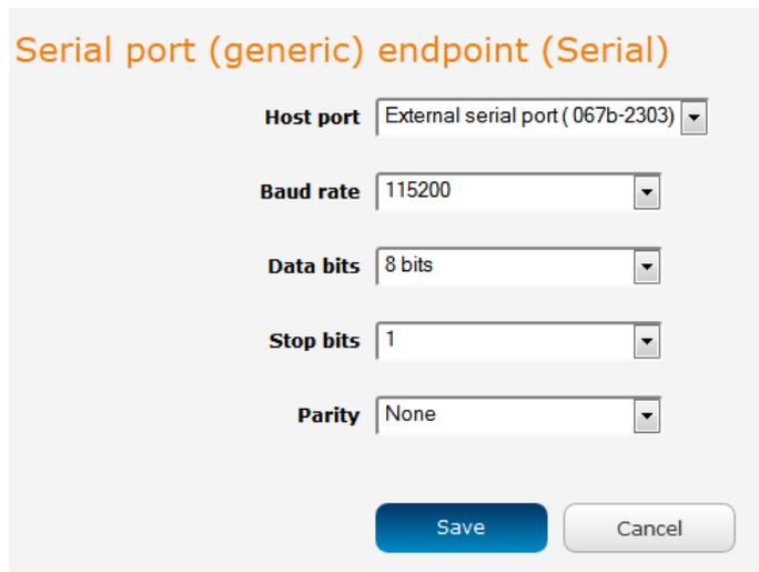
Figure 88 - Serial port (generic) endpoint configuration
