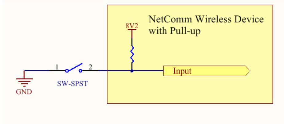
The following input detects an input going high. The turn on/off threshold can be set in the software.
