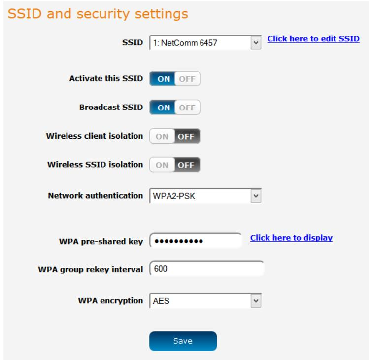
Figure 43 - Wireless Settings – SSID and Security Settings
