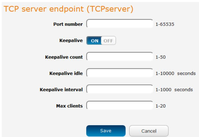
Figure 89 - TCP server endpoint configuration
