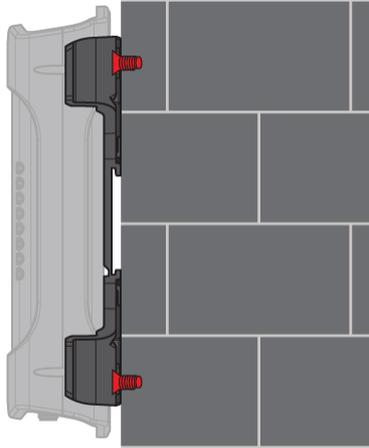
*Figure 7 - Wall mounted via DIN rail bracket*
