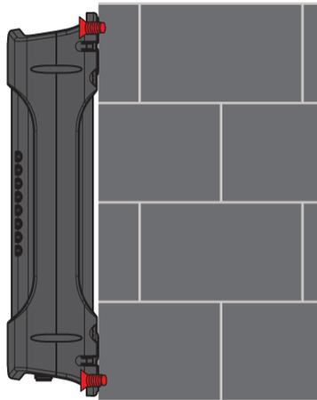
*Figure 5 - Wall mount - Flat against the wall*
