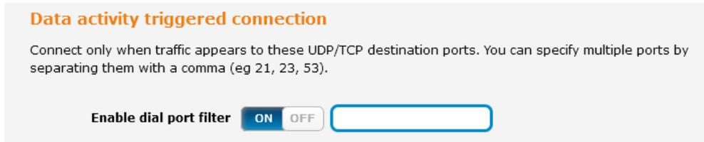
Figure 20 – Connect on demand - Data activity triggered connection
