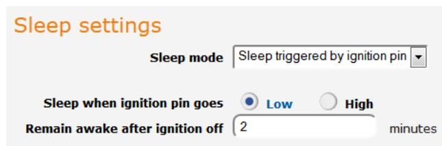
The screenshot shows the 'Sleep settings' section with the 'Sleep mode' dropdown set to 'Sleep triggered by ignition pin'. Below it, there are two radio buttons for 'Sleep when ignition pin goes', with 'Low' selected. At the bottom, the 'Remain awake after ignition off' field contains the number '2' and is followed by the text 'minutes'.
