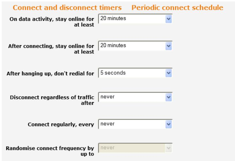
Figure 24 – Connect on demand - Connect and disconnect timers
