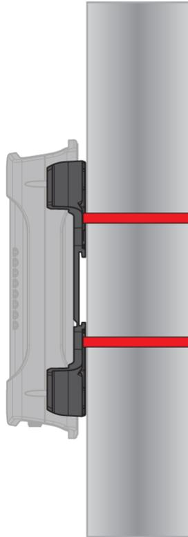
*Figure 9 - Pole mount using DIN rail bracket*
