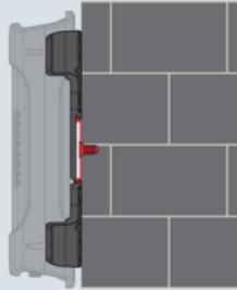
Pole mount using DIN Rail bracket
