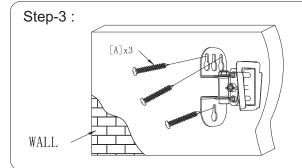
Fix the wall dead plate with six lag bolts to install the wall fixed installation for the panel TV on the vertical wall
