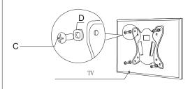
Install the panel TV on the TV fixed plate with suitable bolts.
