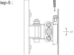
Hang the TV fixed plate in connection with the TV panle on the wall dead plate. At last adjust the azimuth of the panel TV to a suitable position for watching.
