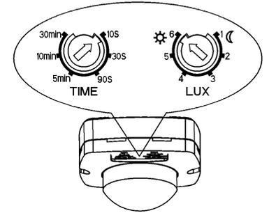
Please note that when testing in daylight, turn the LUX selector to the ☀ (SUN) position, otherwise the sensor will not turn on the load. Also ensure that any lamp connected as a load is pointed away from, and is mounted no closer than 60cm from the sensor.
