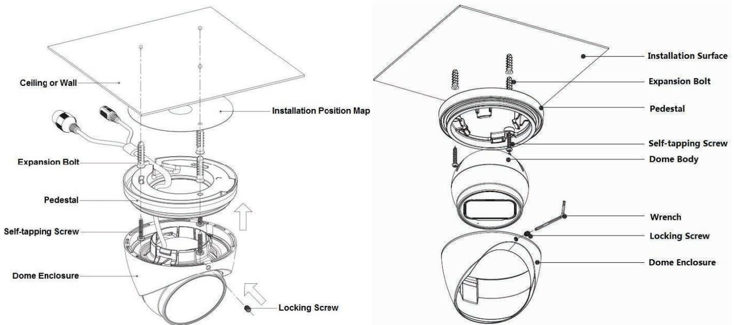
1. Position the installation map to a wall or ceiling and drill holes where marked.
