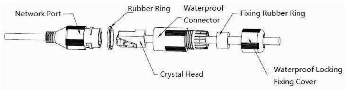
1. Install the rubber ring into the network port, keeping the smaller hole of the rubber ring facing outwards and fixing the rubber ring onto the main body of the waterproof cable.
