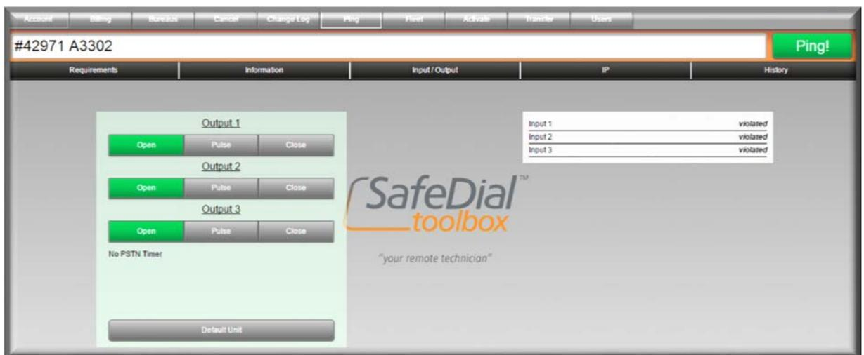
The outputs can be opened, closed and pulsed.
