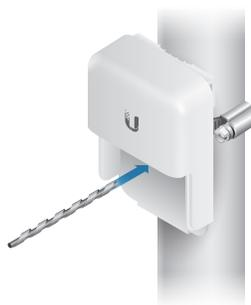
2. Drill a pilot hole into the pole.
