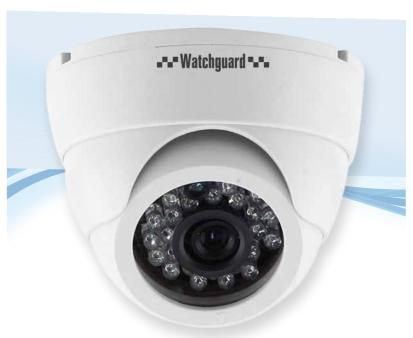
The Watchguard VSDFF20MIR800VPV2 is a stylish dome camera capable of streaming beyond 800TVL definition footage. This camera features up to 800TVL image resolution, with 20m infrared range for low light/night video capture and a standard 3.6mm fixed lens. The camera housing is IP66 rated, making it suitable for outdoor surveillance.
