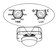
Turn LUX selector anti-clockwise to the minimum setting (moon). If the ambient light is more than three lux, the load will not turn back on after the sensed movement has stopped.
