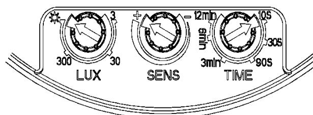
Note: When testing in daylight, please turn LUX knob to the maximum setting (SUN) to allow the sensor to work.
