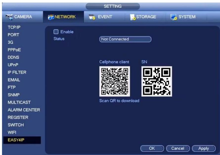
7. Ensure "Enable" is ticked. Then select the "Apply" button. The "Status" will change to "Connect Success" once the recorder has a connection to the P2P server. This normally takes 1 minute.
