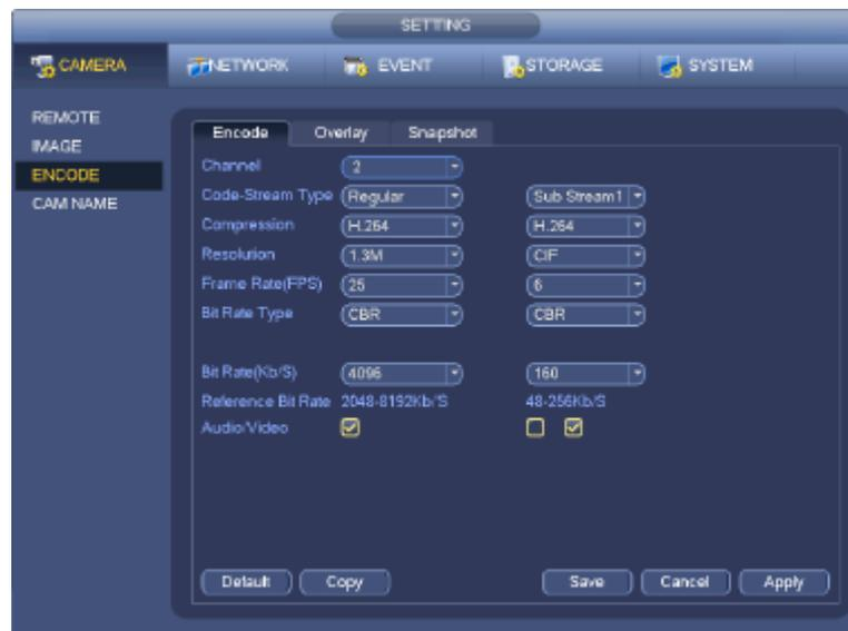
In this menu, you can set individual encoding options for Regular, Motion Detect and Alarm Recording.
