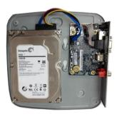
6 Connect the HDD cable and power cable.
