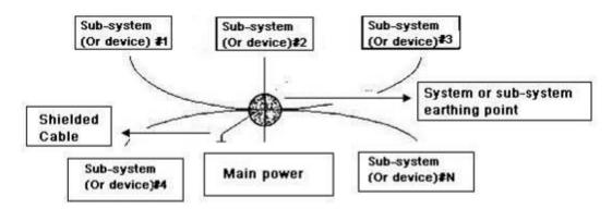
Multiple-point ground: In the following figure, you can see the internal circuit uses the chassis as the common point. While at the same time, all devices chassis use the earthing as the common port. In this connection, the ground structure can provide the lower ground resistance because when there are multiple-point grounds; each ground cable is as short as possible. And the parallel cable connection can reduce the total
