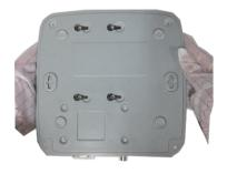
4 Turn the device upside down and 5 Fix the HDD firmly. then turn the screws in firmly.
