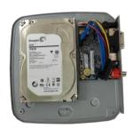
3 Place the HDD in accordance with the four holes in the bottom.
