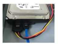
5 Connect the HDD cable and power cable.
